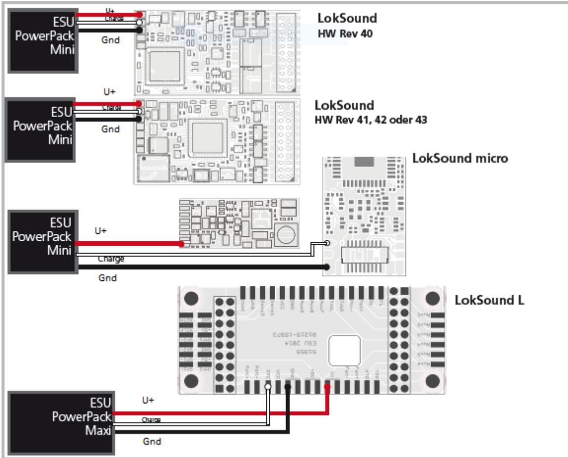
If using a 2 wire Power Pack connect as shown:
