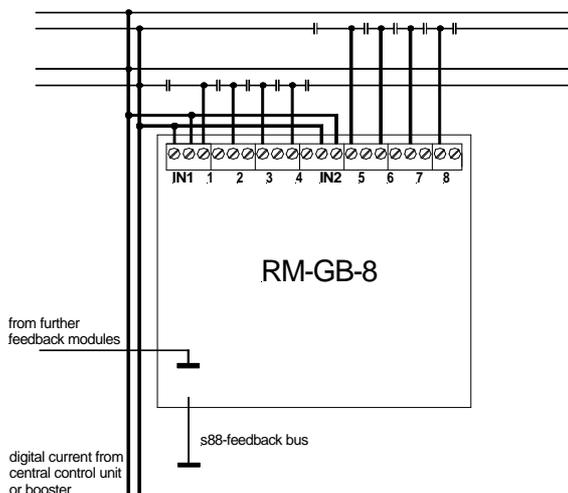
Digital current will be supplied to the **RM-GB-8** via input **IN1** and **IN2**. **IN1** provides current to the output **1** to **4** and **IN2** provides current to the out put **5** to **8**. The two inputs **IN1** and **IN2** are **electrical separated**. Therefore it will be possible for
