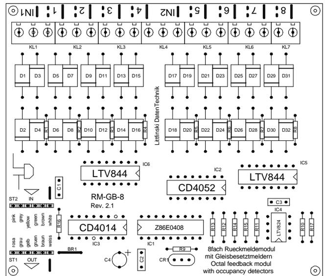
The **track voltage** and the **feedback bus** are separated by **optogalvanic**. The current for the tracks can therefore safely be supplied from different transformers without having a negative effect on the digital control units.
